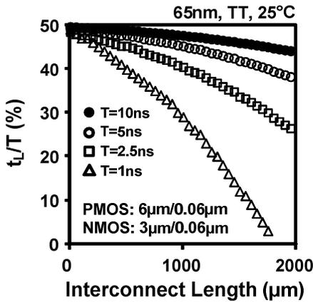
Figure 9. Normalized duty cycle for which the PMOS is deeply biased on decreases with a longer interconnect due to the decreased slew rate.
