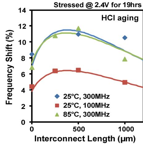
Figure 10. Measured data (in markers) and aging model proposed in section IV-C (curves) for HCI induced frequency degradation.
