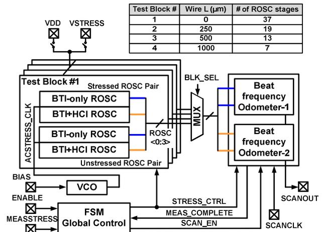
Figure 1. Interconnect odometer test chip diagram. Four ROSCs (stressed pair and unstressed pair) are used for each wire configuration to separately monitor BTI and HCI induced frequency shifts.
