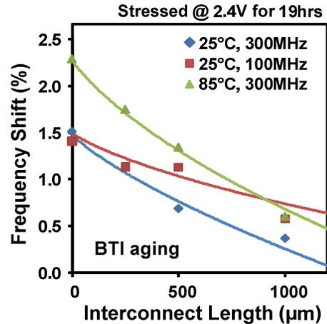
Figure 7. Measured data (in markers) and aging model proposed in section IV-B (curves) for BTI induced frequency degradation.
