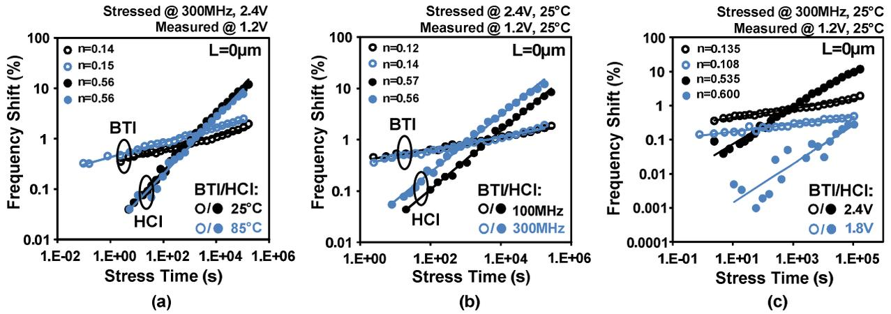
Figure 5. Measured BTI and HCI contribution under different (a) temperatures, (b) frequencies, and (c) stress voltages. The HCI component is obtained by subtracting out the BTI-only degradation from the BTI+HCI degradation.
