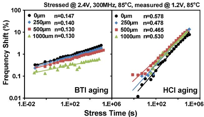
Figure 6. Measured frequency degradation induced by BTI and HCI for different interconnect lengths. BTI is the worst at L=0µm (left) while HCI is worst at L=500µm (right).
