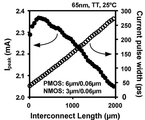
Figure 12. HCI parameters versus interconnect length. NMOS peak current decreases with interconnect length, while the pulse width increases. The combined effect is a non-monotonic dependence of HCI induced frequency degradation on interconnect length.
