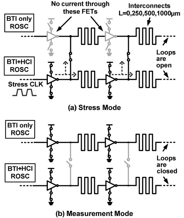
Figure 3. ROSC pair configuration in stress and measurement modes. The top ROSC exhibits the same amount of BTI as the bottom ROSC but without any HCI [5].
