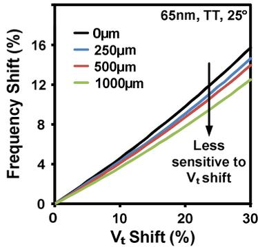
Figure 13. Frequency shift vs.  $V_t$  shift for different interconnect length. The frequency shift of a interconnect dominated signal path is less sensitive to the logic device aging due to the invariant wire RC delay. This is captured using the sensitivity factor parameter shown in section IV-A.
