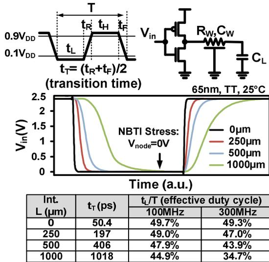
Figure 8. Effective stress time ( $t_t$ ) decreases in longer interconnects resulting in a smaller BTI degradation as shown in Fig. 7.
