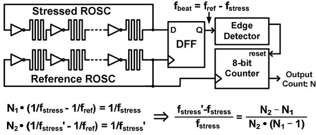
Figure 2. Beat frequency odometer system used in this work.  $N_1$  and  $N_2$  are the counts from the counter output, recorded before and after a certain stress period. Using the equations listed above, we can conveniently calculate the percentage frequency change with picosecond level precision.
